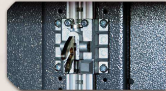
Drawer pull-out interlock system.
